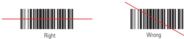
**Figure 2-17** Laser Scanner Aiming Pattern
