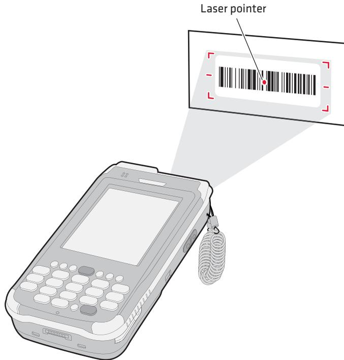
**4** When a bar code label is successfully read, the CN3 makes a high beep and the Good Read LED lights briefly.
