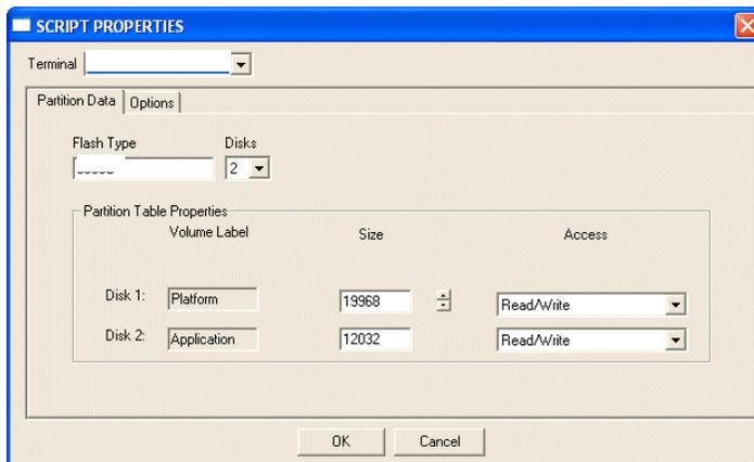
**Figure 6-2** *Script Properties* Window - *Partition Data* Tab
