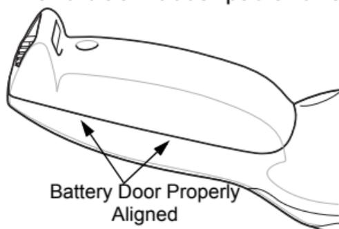
11. Secure the battery cover with the Torx screw using a T8 Torx drive.
