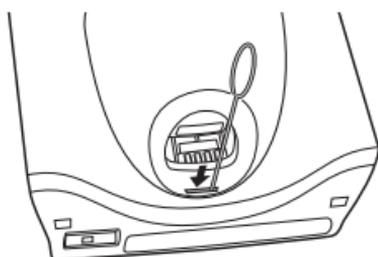
6. While holding the key down, lift the mobile computer out of the cradle.
