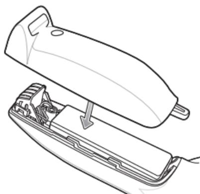
10. Inspect the position of the battery cover with the main housing. If the door is misaligned, remove battery and black rubber pad and re-install.
