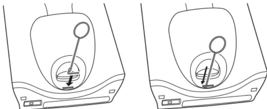
3. Slide the key to the right until the handle is centered in the slot.
