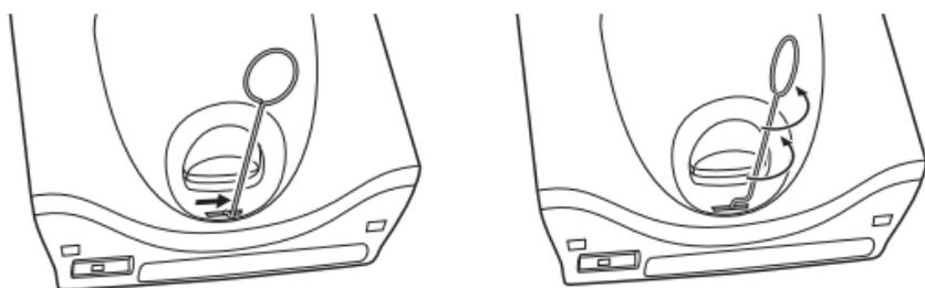
5. Keeping the handle of the key all the way to the right in the slot, press the key into the slot. The end of the key should press on a small spring loaded tab within the cradle.
