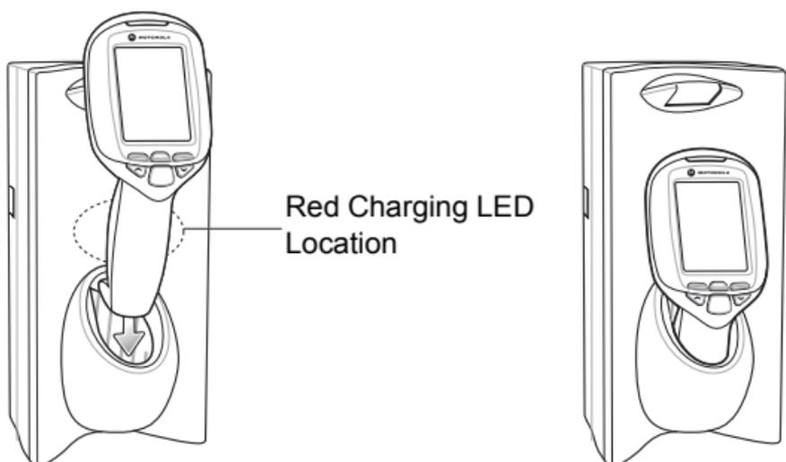
3. The mobile computer starts to charge automatically. The mobile computer fully charges in approximately five hours. While charging, a red charging LED can be seen through the front panel of the cradle behind the mobile computer. Refer to the MC17 *Product Reference Guide* for specific charging profile information.
