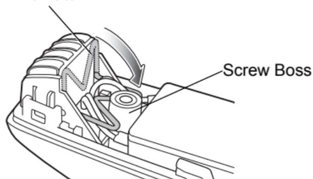
9. Place the battery cover onto the handle and slide it as shown.
